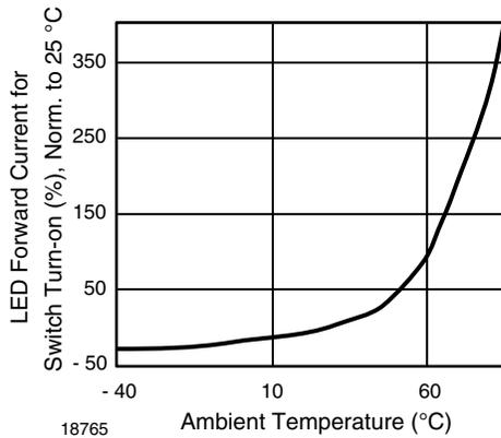
Fig. 18 - LED Current for Switch Turn-on vs. Temperature
