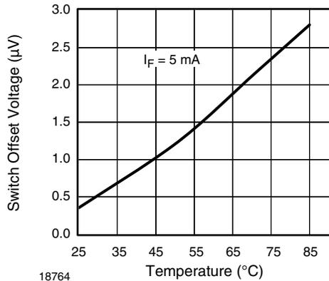
Fig. 17 - Switch Offset Voltage vs. Temperature
