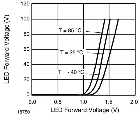
Fig. 3 - LED Forward Current vs. LED Forward Voltage
