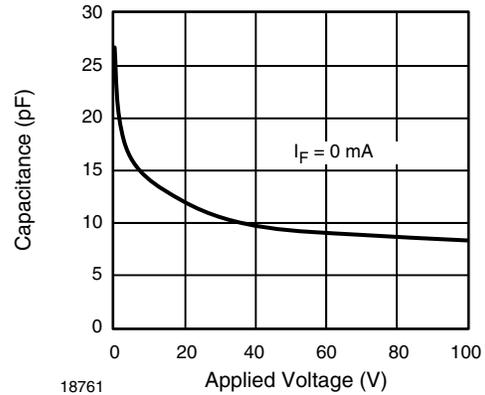
Fig. 14 - Switch Terminal Capacitance vs. Applied Voltage
