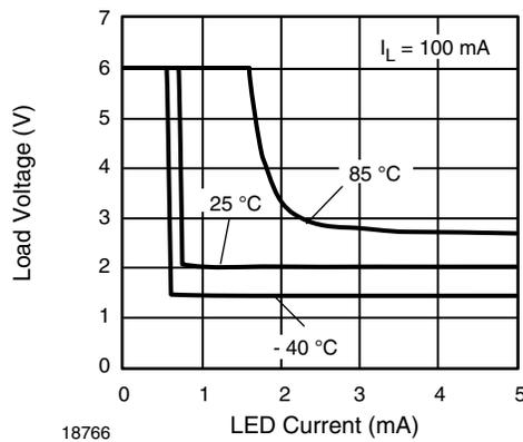
Fig. 19 - LED Current vs. Load Voltage
