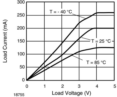
Fig. 8 - Load Current vs. Load Voltage
