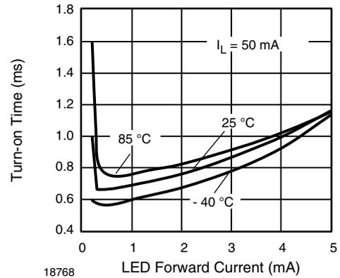
Fig. 21 - Turn-on Time vs. LED Current
