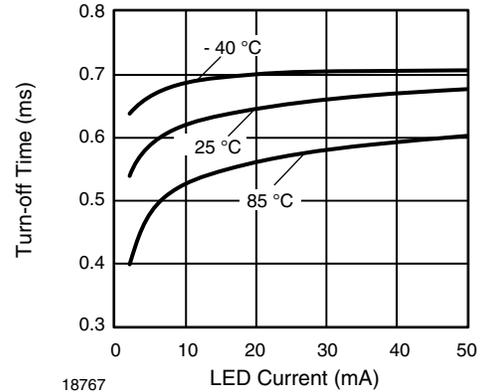
Fig. 20 - Turn-off Time vs. LED Current
