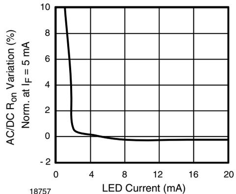
Fig. 10 - Variation in On-resistance vs. LED Current
