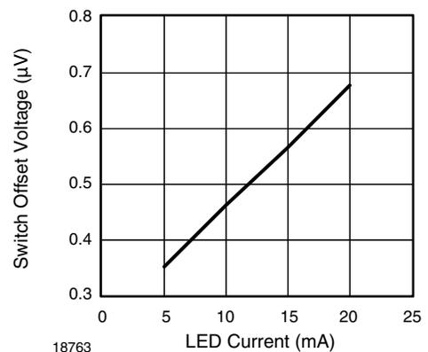
Fig. 16 - Switch Offset Voltage vs. LED Current
