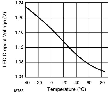
Fig. 11 - LED Dropout Voltage vs. Temperature
