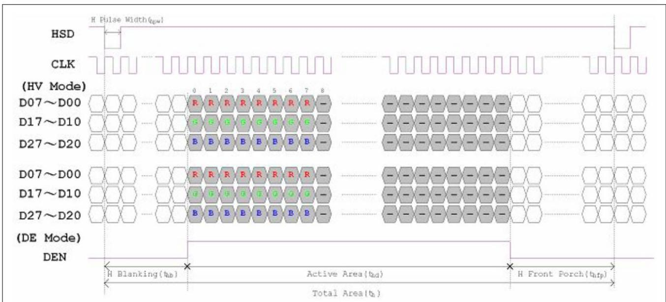
Figure 6.1: Clock and Data Input Timing Diagram
