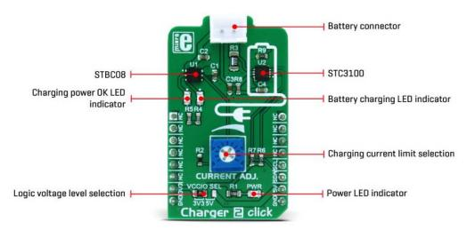
Two LEDs are used to signalize status of the STBC08 IC: red LED is used to signalize the ongoing charge process. The green LED signalizes if the charging conditions are nominal and within the specs. It signalizes the validity of the charging voltage value.
