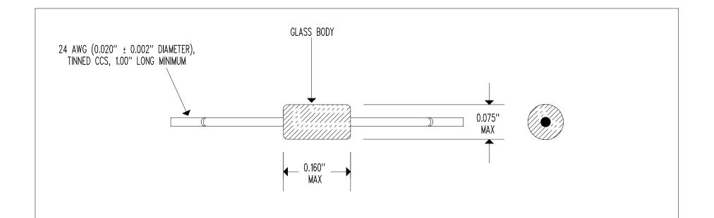
RESISTANCE @  $+25^{\circ}C = 220,000 \Omega \pm 10\%$ RESISTANCE/TEMPERATURE CURVE = "J" TEMPERATURE COEFFICIENT @  $+25^{\circ}C = -4.4\%$ 'C NOMINAL BETA " $\beta$ " (0 TO  $+50^{\circ}C$ ) = 3,892'K NOMINAL DISSIPATION CONSTANT = 2 mW/'C NOMINAL (STILL AIR) THERMAL TIME CONSTANT = 5 SECONDS NOMINAL (STILL AIR) THERMAL TIME CONSTANT = 0.5 SECONDS NOMINAL (STIRRED OIL) MAXIMUM TEMPERATURE RATING =  $+300^{\circ}C$
