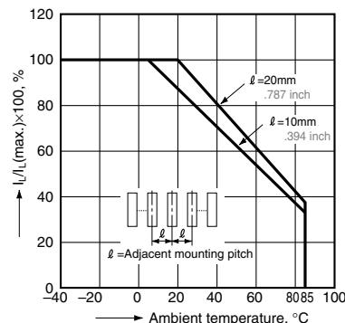
3. On resistance vs. ambient temperature characteristics
