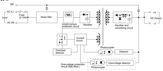
Note: Only the S8E1 with an output of 5 V incorporates an overvoltage protection circuit.
