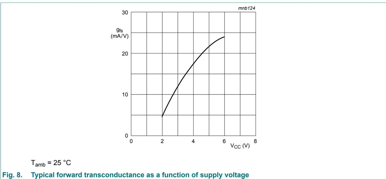
Fig. 8. Typical forward transconductance as a function of supply voltage
