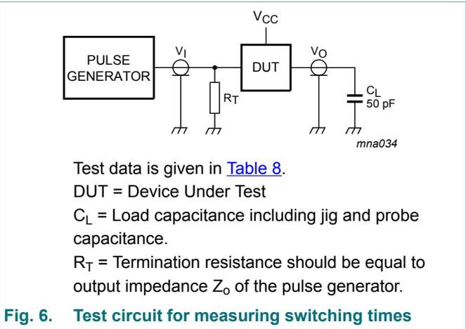
Fig. 6. Test circuit for measuring switching times
