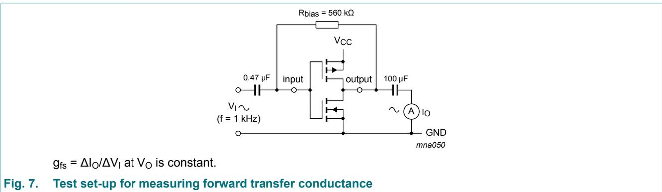
Fig. 7. Test set-up for measuring forward transfer conductance
