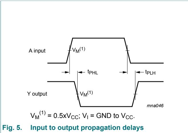
Fig. 5. Input to output propagation delays
