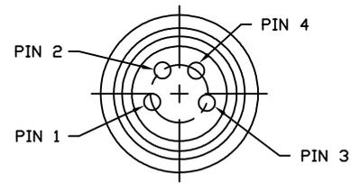
WHEN MATING WITH NORCOMP CONNECTORS, ONLY AN IP66 RATING CAN BE ACHIEVED IN MATING AREA BETWEEN CONNECTORS. CONNECTOR IS OTHERWISE IP67 AND MAY BE FULLY IP67 IF MATED WITH COMPETITOR PARTS.
