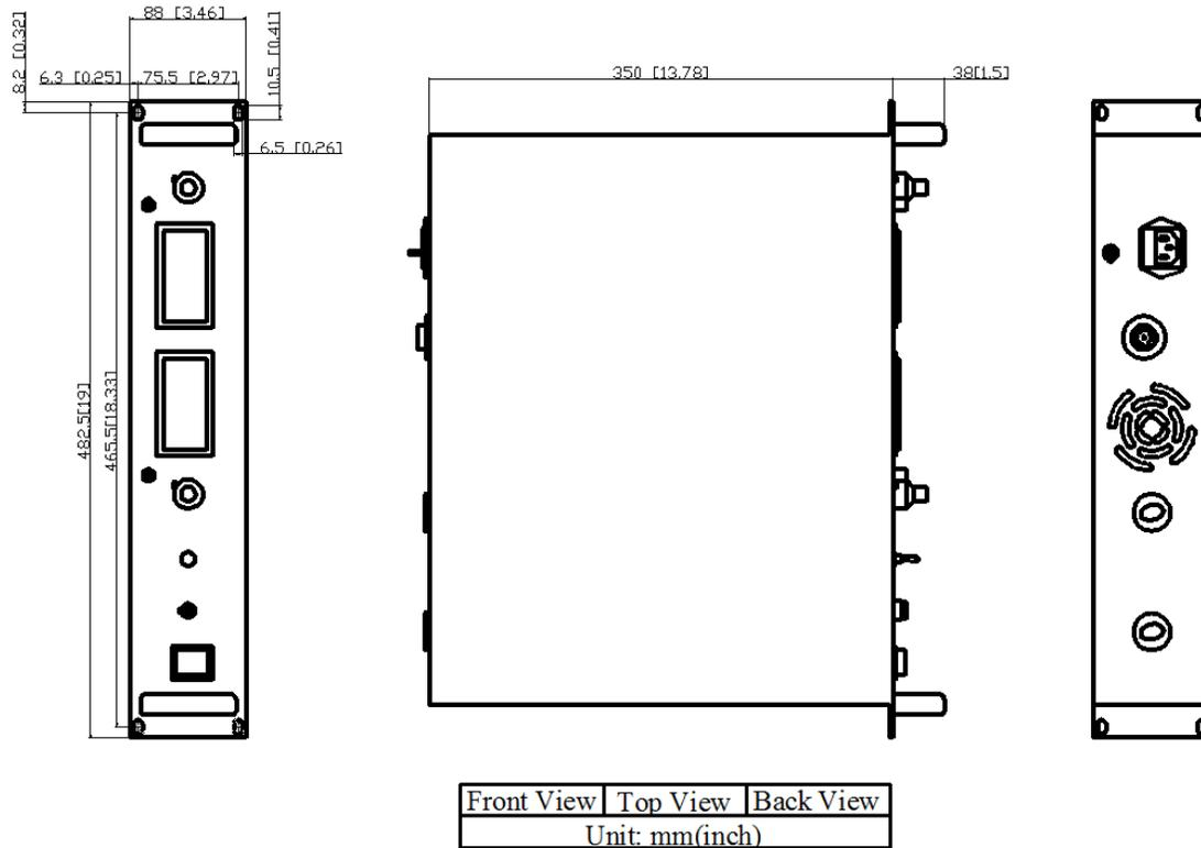
Figure 9. Dimensions for A2UHVAC3KV50MAIRM
