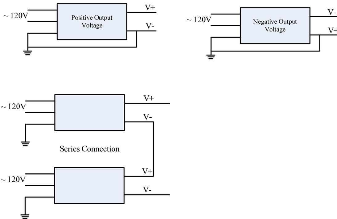
Figure 7. Wiring Connection
