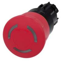
Illum. emergency stop mushroom pushbutton, 22 mm, round, plastic, red, 40mm, positive latching, rotate-to-unlatch, with laser labeling, upper case and lower case, always upper case at beginning of line
