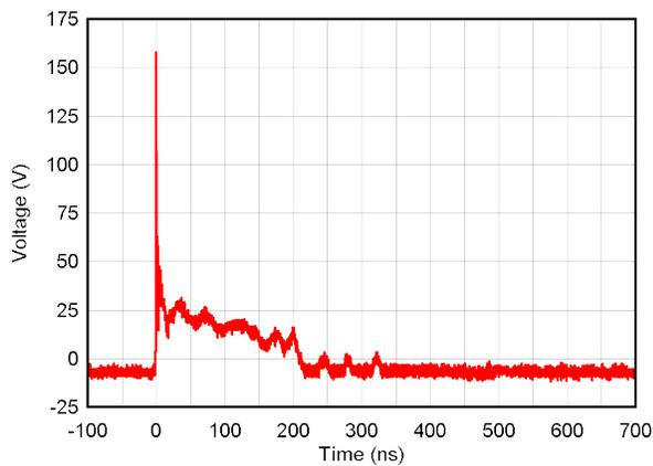
Figure 7-3. +8-kV Clamped IEC Waveform
