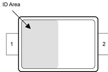
**Figure 5-1. DYF Package, 2-Pin SOD-323 (Top View)**
