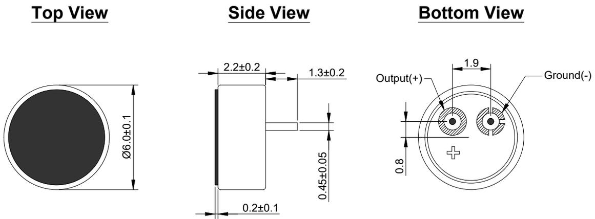
Figure 4. HBO0603B-52/1338 Mechanical Layout
