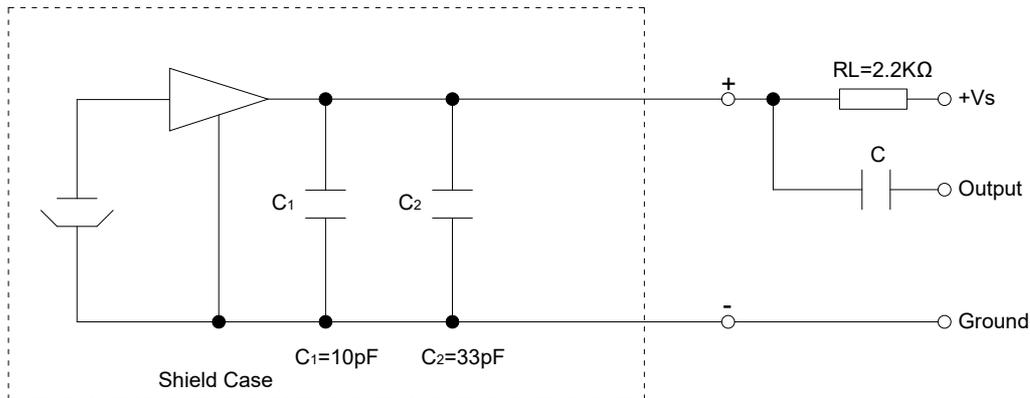
Figure 3. Schematic Diagram
