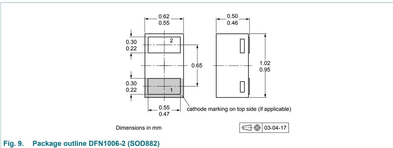
Fig. 9. Package outline DFN1006-2 (SOD882)
