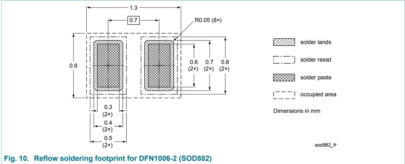
Fig. 10. Reflow soldering footprint for DFN1006-2 (SOD882)
