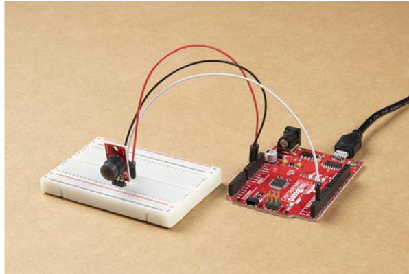
If you are using a Raspberry Pi or other SBC/development-board that uses Python as its primary programming language, follow the above assembly steps for the PIR and connect it to your Pi/SBC's GPIO header taking care to make the proper pin connections. Raspberry Pi users looking for a quick GPIO reference can find one here or you can use the `pinout` command from the GPIO Zero Python Library in the console to display the pinout there.
