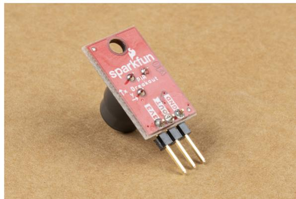
Next, we plug the sensor into the breadboard (users connecting directly to their microcontroller can ignore this step) taking care to orient it properly so the pins are not sharing the same rail. After the PIR is in place, select three jumper wires and connect the PIR's pins to the matching pins on the microcontroller. **3.3V** to **3.3V**, GND to Ground/GND and OUT to a digital I/O pin.
