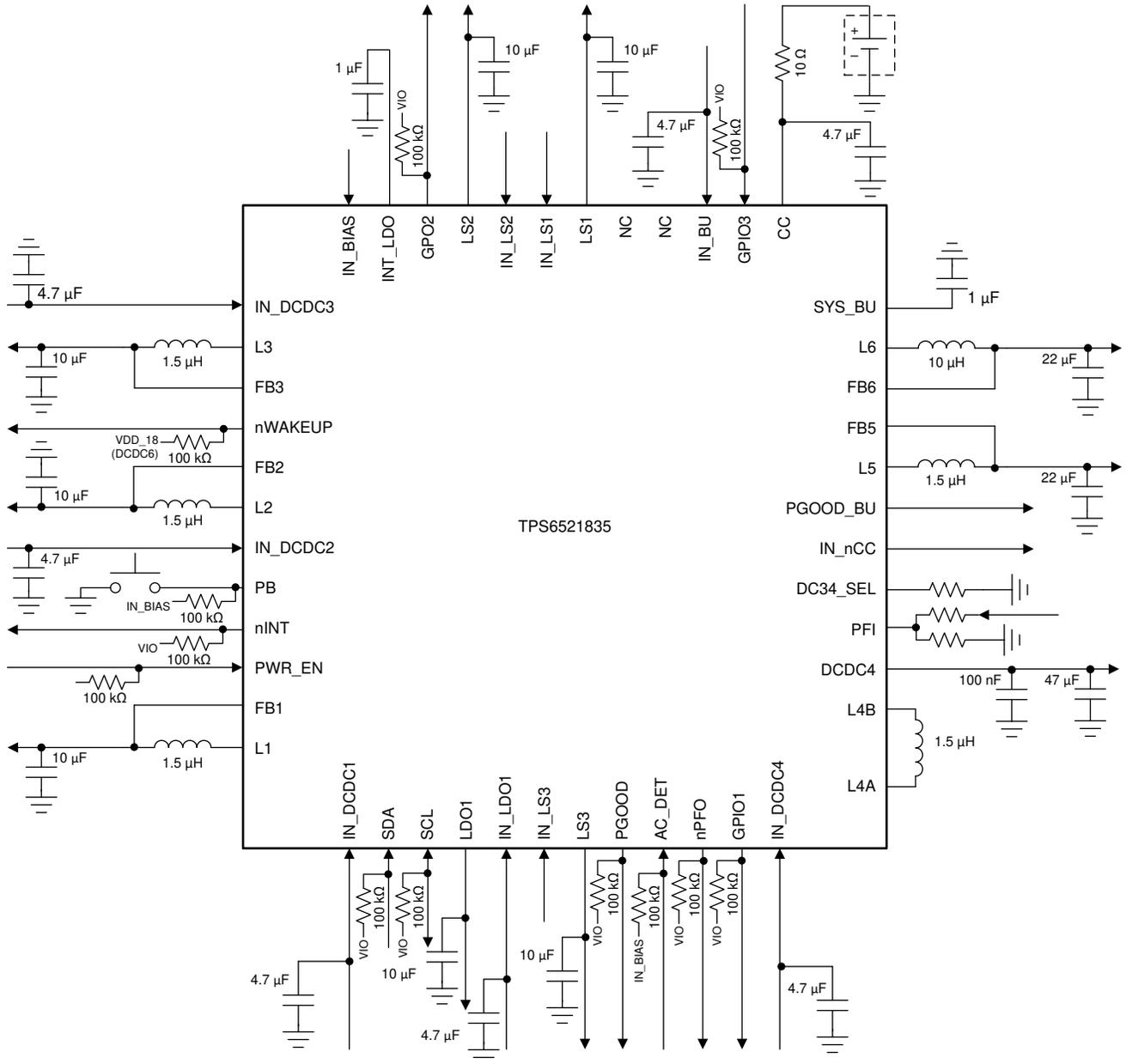
Figure 3-1. Simplified Schematic
