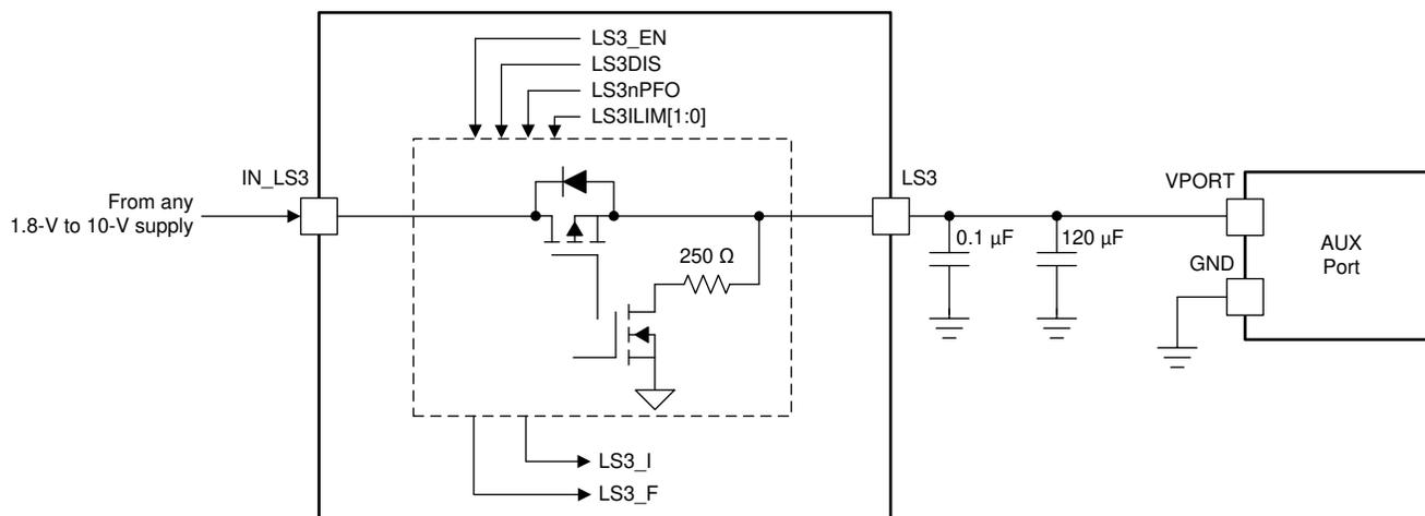
**Figure 7-13. Typical Application of Load Switch 3**
