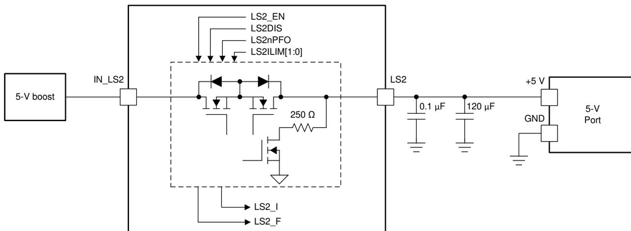
**Figure 7-12. Typical Application of Load Switch 2**
