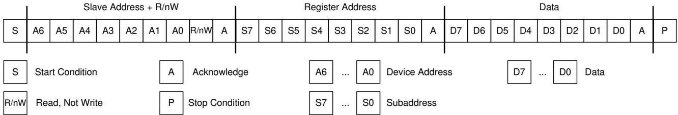
**Figure 7-31. Subaddress in I<sup>2</sup>C Transmission**
