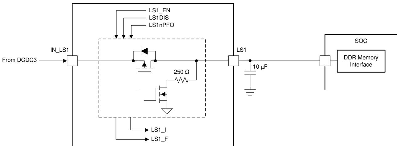
Figure 7-11. Typical Application of Load Switch 1
