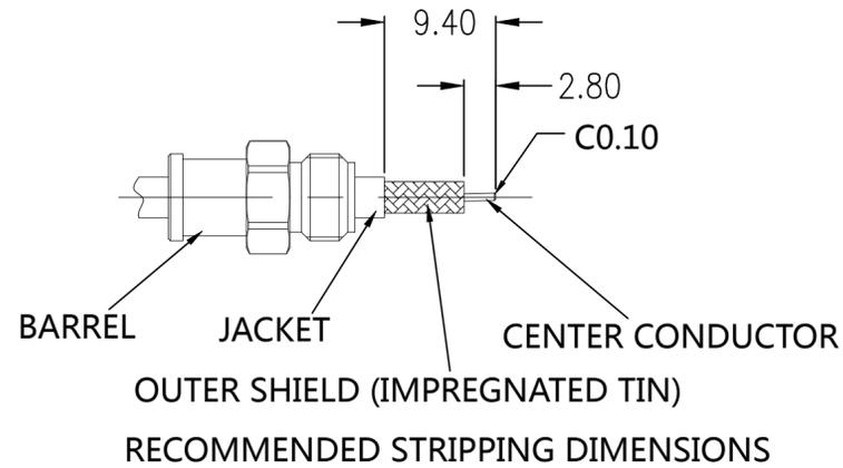
2. A. As shown in the left figure, put the welding cup on the outer shielding layer of the cable first.
