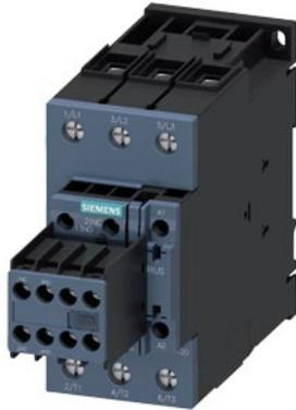
power contactor, AC-3 40 A, 18.5 kW / 400 V 2 NO + 2 NC, AC / DC 20-33 V, with varistor, 3-pole, Size S2, screw terminal
