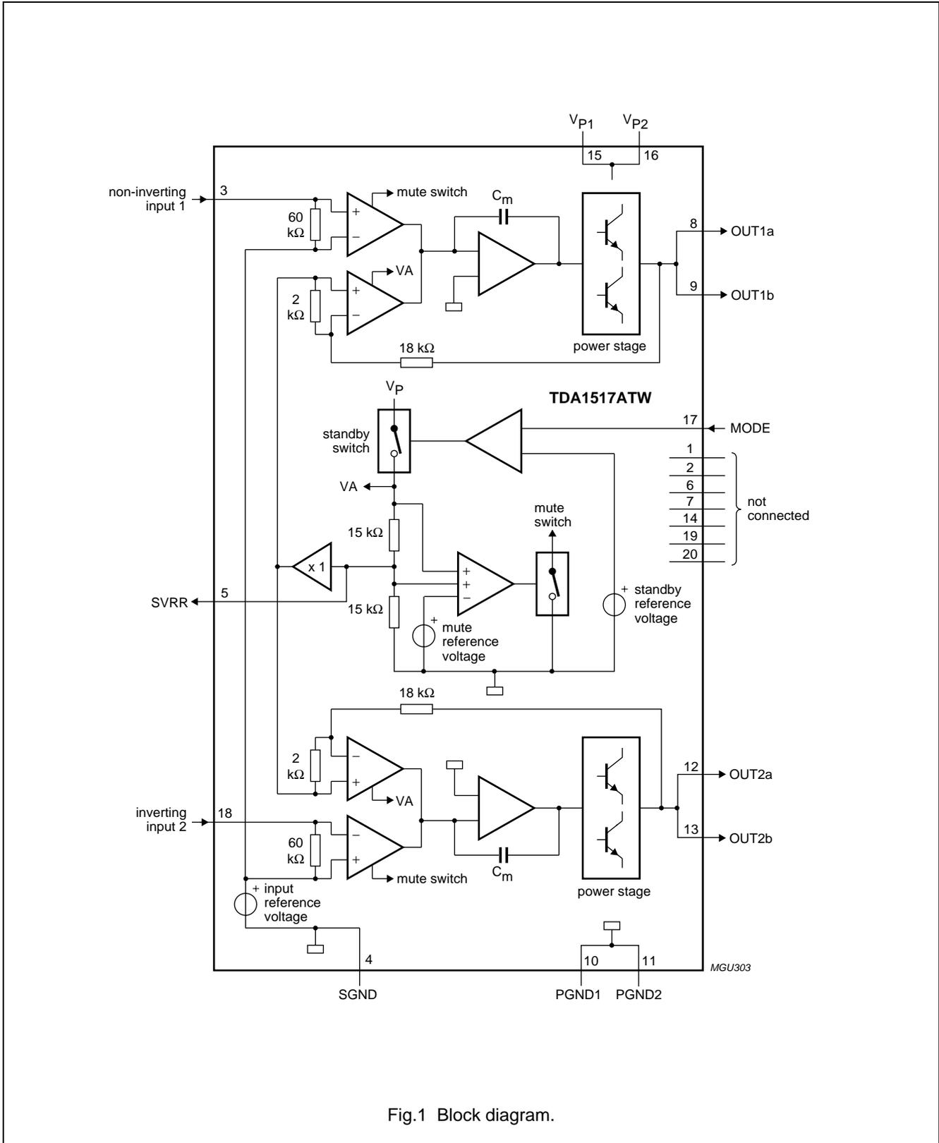
Fig.1 Block diagram.
