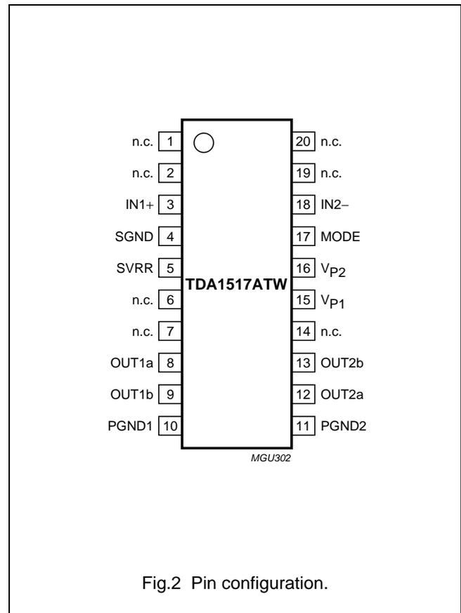
Fig.2 Pin configuration.
