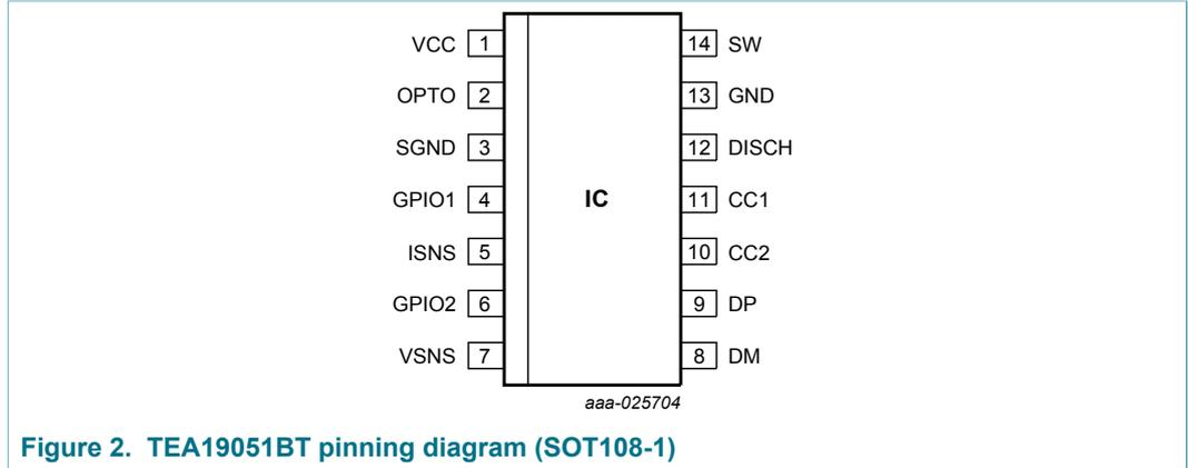
Figure 2. TEA19051BT pinning diagram (SOT108-1)
