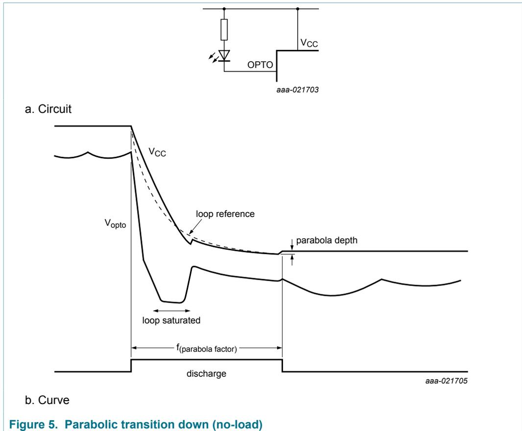
Figure 5. Parabolic transition down (no-load)
