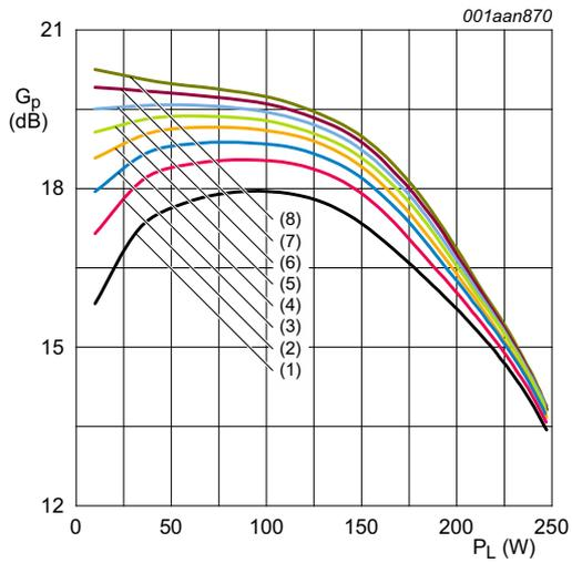
$V_{DS} = 50 \text{ V}$ ;  $f = 1300 \text{ MHz}$ ; carrier spacing = 100 kHz.
