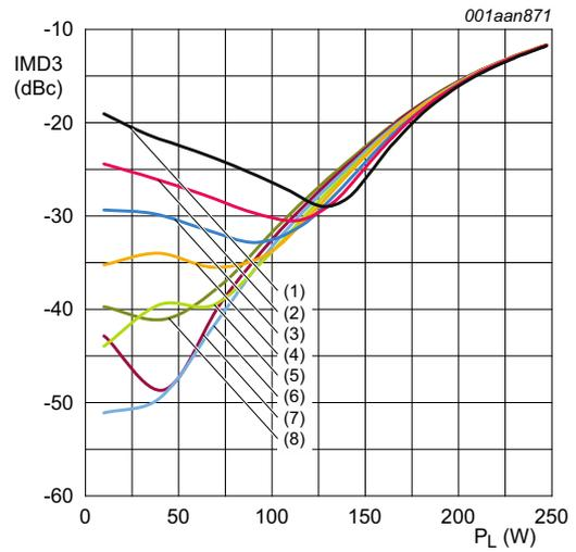
$V_{DS} = 50 \text{ V}$ ;  $f = 1300 \text{ MHz}$ ; carrier spacing = 100 kHz.
