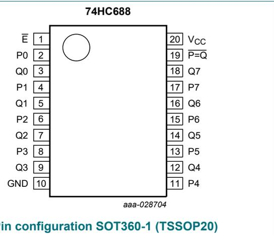
Fig. 5. Pin configuration SOT360-1 (TSSOP20)
