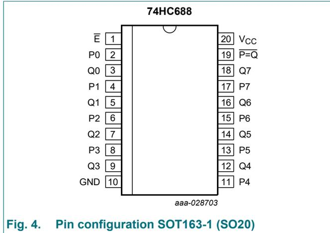
Fig. 4. Pin configuration SOT163-1 (SO20)
