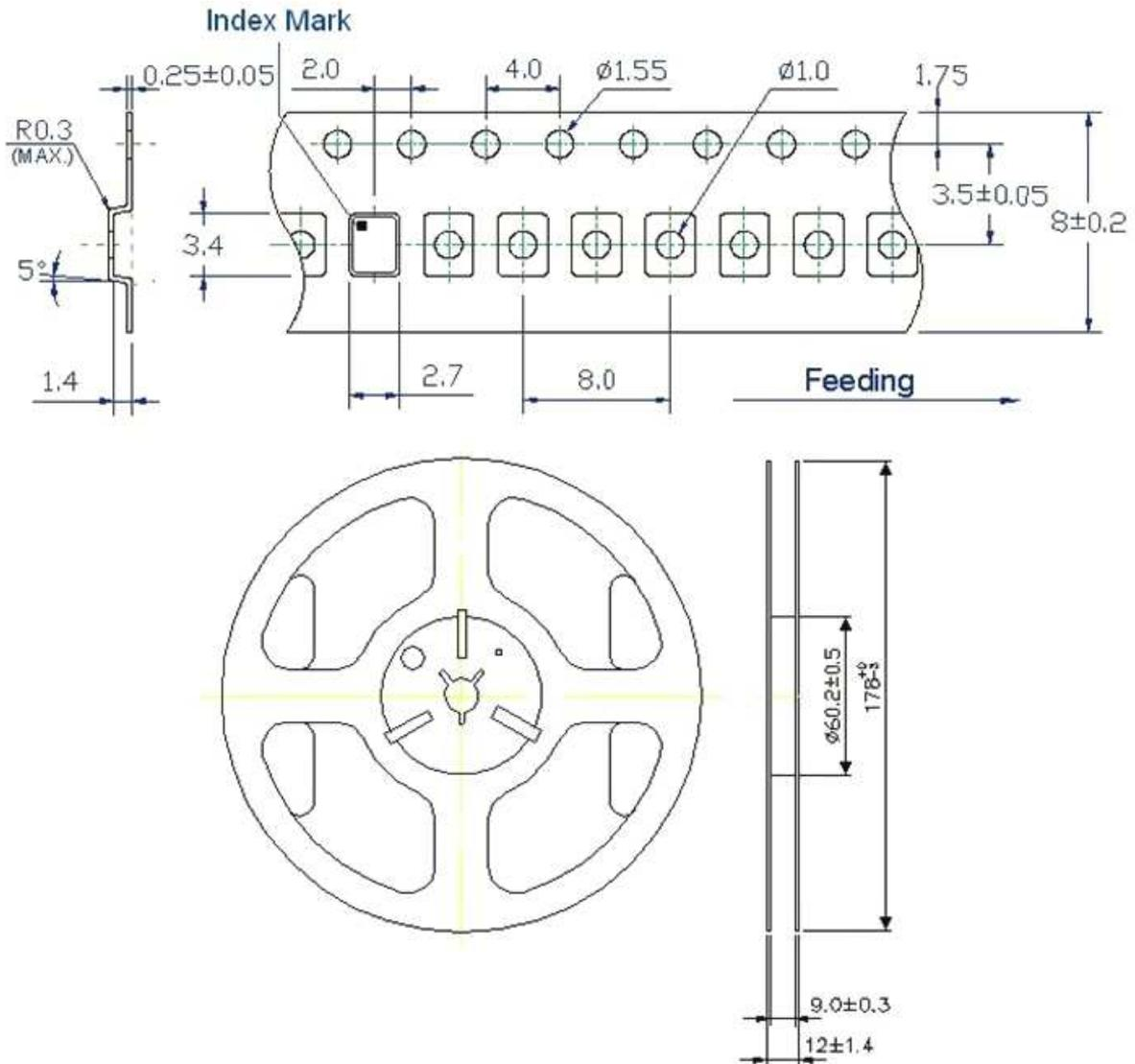
1. 230mm minimum leader which consist of carrier and/or tape followed by a minimum of 160mm of empty carrier tape sealed with cover tape.
