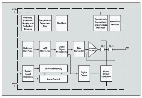
Fig. 2: Block diagram of the HAC 830
