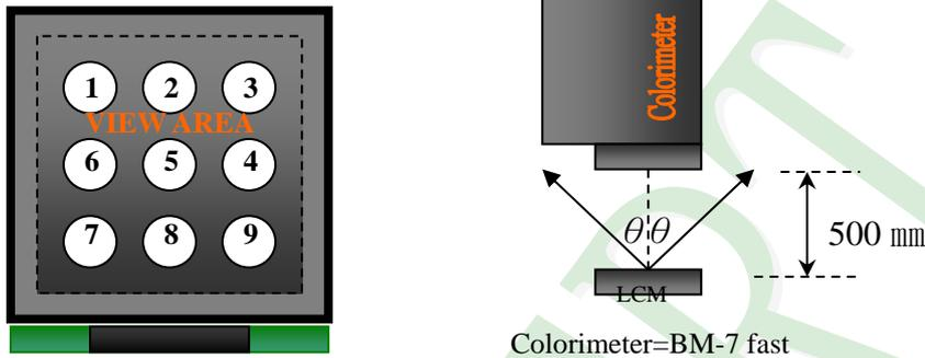
To be measured at the center area of panel with a viewing cone of  $1^{\circ}$  by Topcon luminance meter BM-7, after 10 minutes operation (module)
