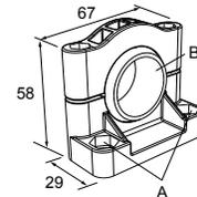
**Hole center spacing:** A=ø 50.8
