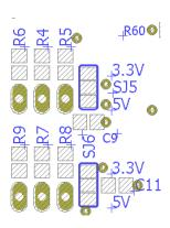
Most external connections to the Teensy are made through three pin connectors, but DIO18 and DIO19 go through a four pin connector and have a slightly different resistor network to accommodate I2C communication and make the pins more flexible.
