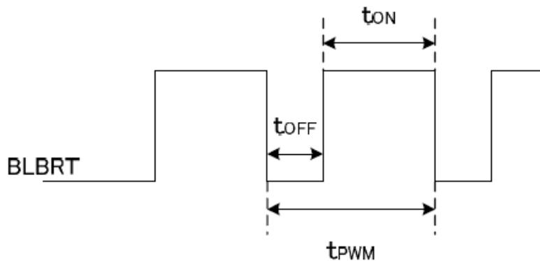
$t_{ON}, t_{OFF} \geq 50 \mu s$ .
