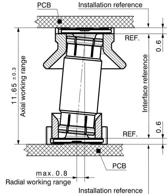
standard MMBX PCB connector without extended pull-in range (e.g. 82 MMBX-S50-0-1)
