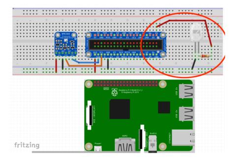
The included 560 Ohm and 10K Ohm resistors will both protect the circuit, the latter make the LED dim. You can sanity check your wiring with python using the following commands one by one:
