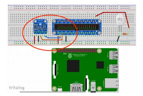
On the Pi Cobbler SDA is data pin and SCL is clock pin. On the BME280 sensor SDI is the data pin and SCK is the clock pin.
