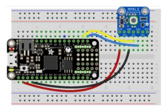
Board 3V to sensor VIN Board GND to sensor GND Board SCL to sensor SCL Board SDA to sensor SDA
