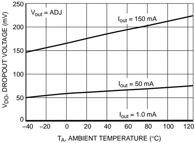
Figure 16. Dropout Voltage vs. Temperature (Over Current Range)
