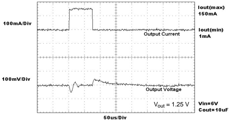
Figure 33. Load Transient Response ( $10\ \mu\text{F}$ )
