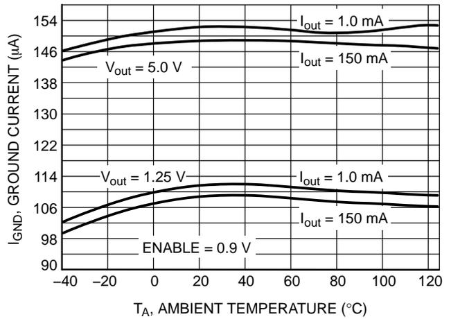
Figure 21. Ground Current (Run Mode) vs. Temperature
