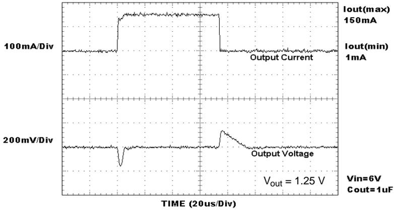
Figure 32. Load Transient Response ( $1.0\ \mu\text{F}$ )
