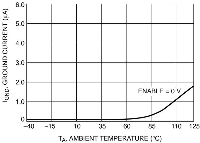
Figure 20. Ground Current (Sleep Mode) vs. Temperature
