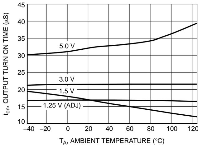
Figure 29. Output Turn On Time vs. Temperature
