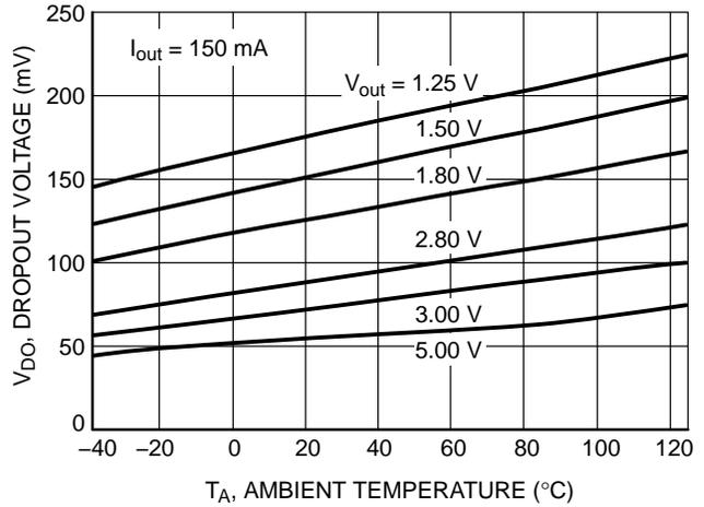
Figure 17. Dropout Voltage vs. Temperature (Over Output Voltage)
