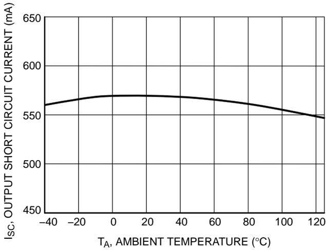
Figure 25. Output Short Circuit Current vs. Temperature
