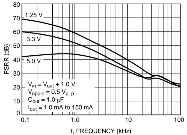
Figure 30. Power Supply Ripple Rejection vs. Frequency
