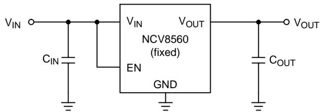
Figure 7. Typical Application Circuit (Fixed Voltage Version)
