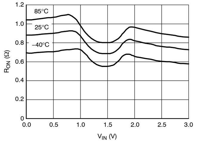
**Figure 8.  $R_{ON}$  vs.  $V_{IN}$  vs. Temperature
