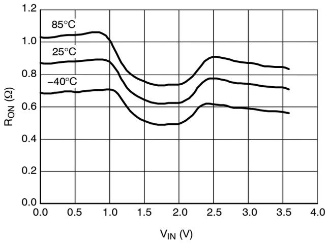
**Figure 9.  $R_{ON}$  vs.  $V_{IN}$  vs. Temperature
