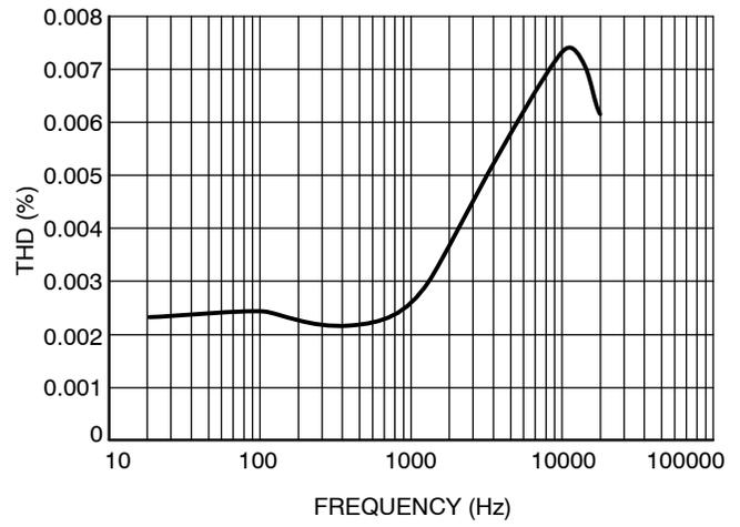
**Figure 10. Total Harmonic Distortion vs.
