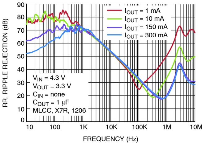
Figure 17. Power Supply Rejection Ratio - C<sub>OUT</sub> = 1 μF
