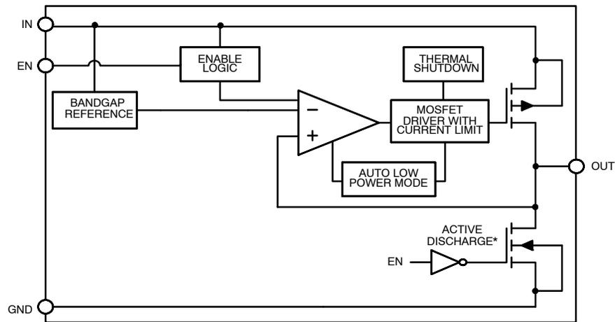
\*Active output discharge function is present only in NCV8114ASNyyyTCG devices. yyy denotes the particular  $V_{OUT}$  option.
