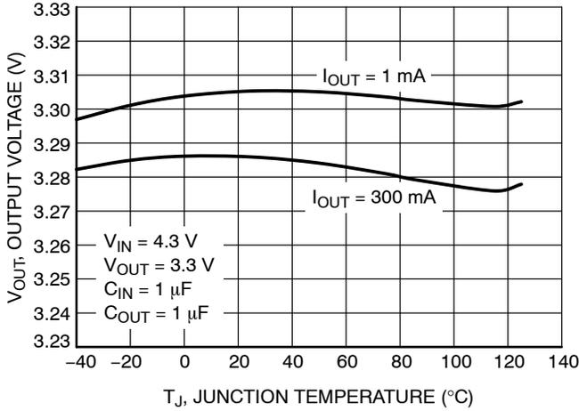
Figure 3. Output Voltage vs. Temperature –  $V_{OUT} = 3.3\text{ V}$
