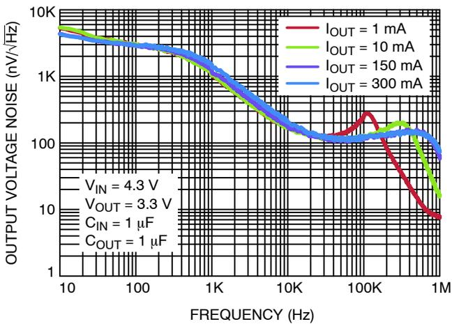
Figure 19. Output Voltage Noise Spectral Density - C<sub>OUT</sub> = 1 μF
