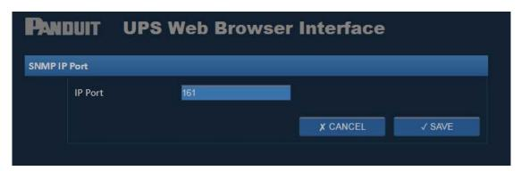
Figure 20: SNMP IP Port Change Pop-up Window
