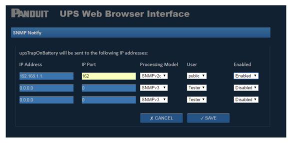
Figure 25: SNMP Trap (Notification) Pop-up Window
