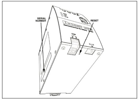
Figure 5: Reset Button and Serial Number
