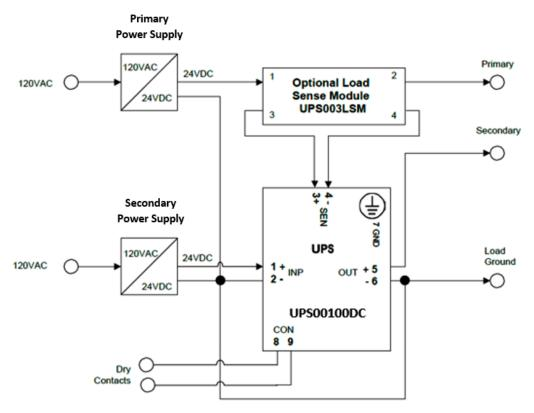
Figure 7: System Wiring Diagram
