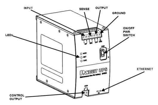
Figure 4: UPS Front Panel Details
