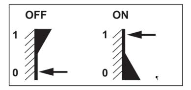
Figure 8: UPS ON/OFF Switch Positions
