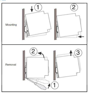
Figure 6: DIN Rail Installation
