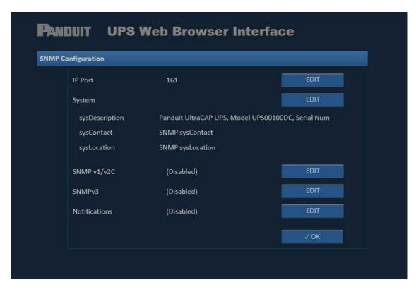
Figure 19: SNMP Configuration Web Page
