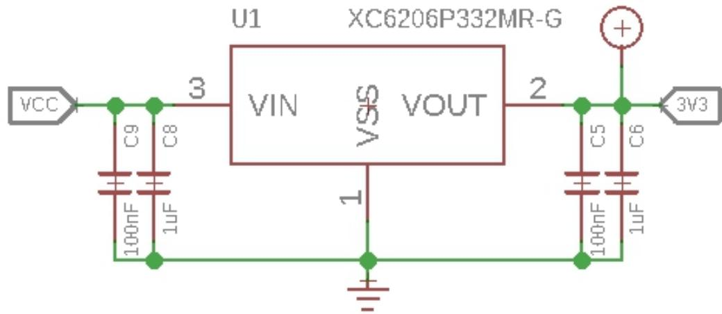
The operating voltage range of MCP9600 is 2.7V ~ 5.5V, we use a power conversion chip XC6206P332MR-G to provide a stable 3.3V for the MCP9600.
