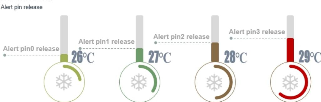
As you can see, there is a hysteresis when the temperature rises and the temperature drops trigger an interrupt. e.g., when the temperature rises, when it reaches 28°C, the alert pin0 will trigger, and when the temperature drops, the limit point becomes 26°C. Only when the temperature become lower than 26 °C, the alert pin0 will release.
