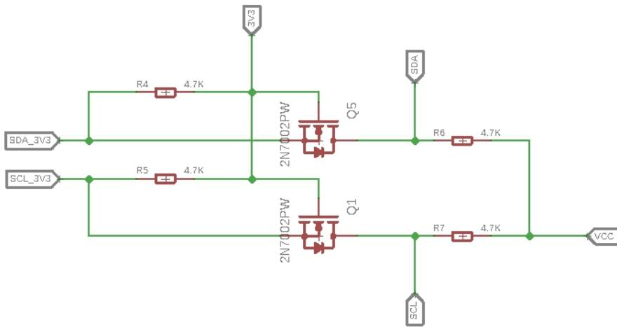
This is a typical Bi-directional level shifter circuit to connect two different voltage section of an I<sup>2</sup>C bus. The I<sup>2</sup>C bus of this sensor use 3.3V, if the I<sup>2</sup>C bus of the Arduino use 5V, this circuit will be needed. In the schematic above, **Q1** and **Q5** are N-Channel MOSFET 2N7002A, which act as a bidirectional switch. In order to better understand this part, you can refer to the AN10441
