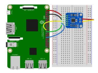
Pi 3.3V to sensor Vin Pi GND to sensor GND Pi SCLK to sensor CLK Pi MISO to sensor DO Pi GPIO 5 to sensor CS
