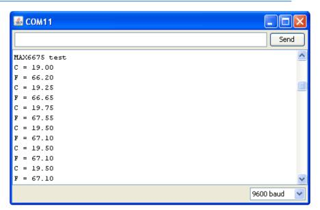
As you can see, its pretty simple to use the library, simply tell the sensor object what the clock, chip select and data pins are, then call readCelsius() or readFahrenheit() to get a floating point result.
