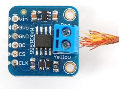
If you're planning to use the MAX6675/MAX31855, there's a little more work to be done. First off, Vin and GND must connect to a 3-5V supply. Then the three data pins must connect to digital IO pins:
