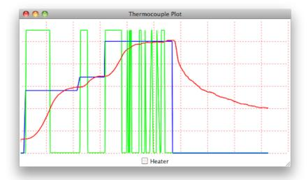
Jeelabs has a detailed walkthrough for a reflow controller (uses an AD595-type chip) (
