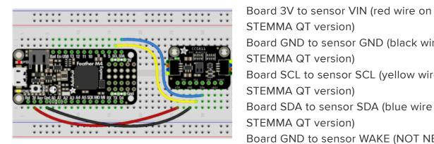
STEMMA QT version) Board GND to sensor GND (black wire on STEMMA QT version) Board SCL to sensor SCL (yellow wire on STEMMA QT version) Board SDA to sensor SDA (blue wire on STEMMA QT version) Board GND to sensor WAKE (NOT NEEDED ON STEMMA QT VERSION)
