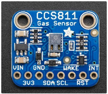
This sensor has 2 mounting holes and one header breakout strip.
