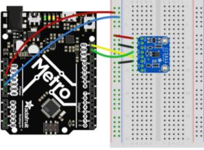
Connect Vin (red wire on STEMMA QT version) to the power supply, 3-5V is fine. Use the same voltage that the microcontroller logic is based off of. For most Arduinos, that is 5V
