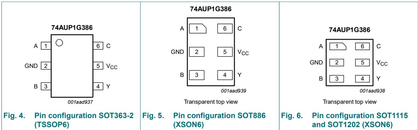
Fig. 4. Pin configuration SOT363-2 (TSSOP6)
