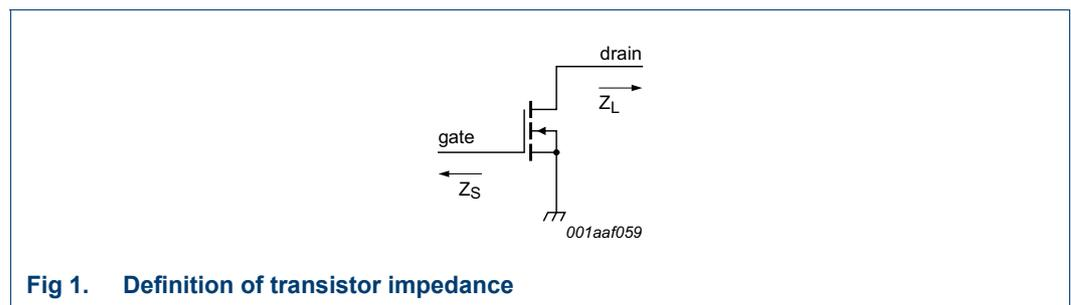
**Fig 1. Definition of transistor impedance**
