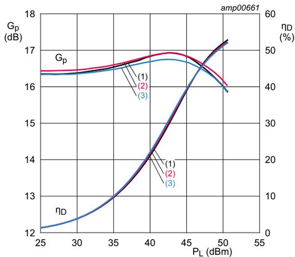
$V_{DS} = 28\text{ V}; I_{Dq} = 800\text{ mA}; V_{GS(amp)peak} = 1.0\text{ V}.$
