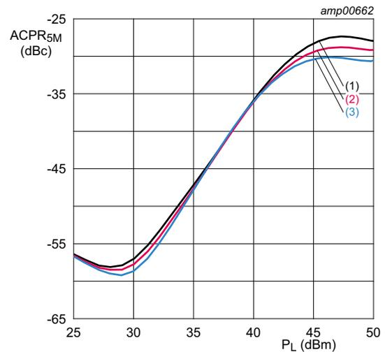
$V_{DS} = 28\text{ V}; I_{Dq} = 800\text{ mA}; V_{GS(amp)peak} = 1.0\text{ V}.$
