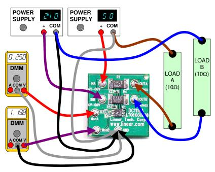
Figure 1. Proper Measurement Equipment Setup
