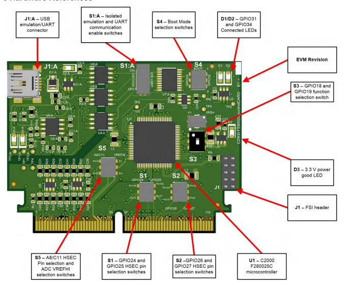
Figure 6-1. Key Components on the controlCARD - Front
