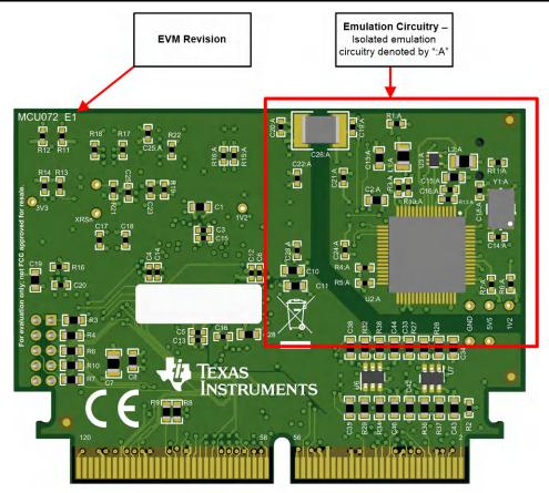
Figure 6-2. Key Components on the controlCARD - Back
