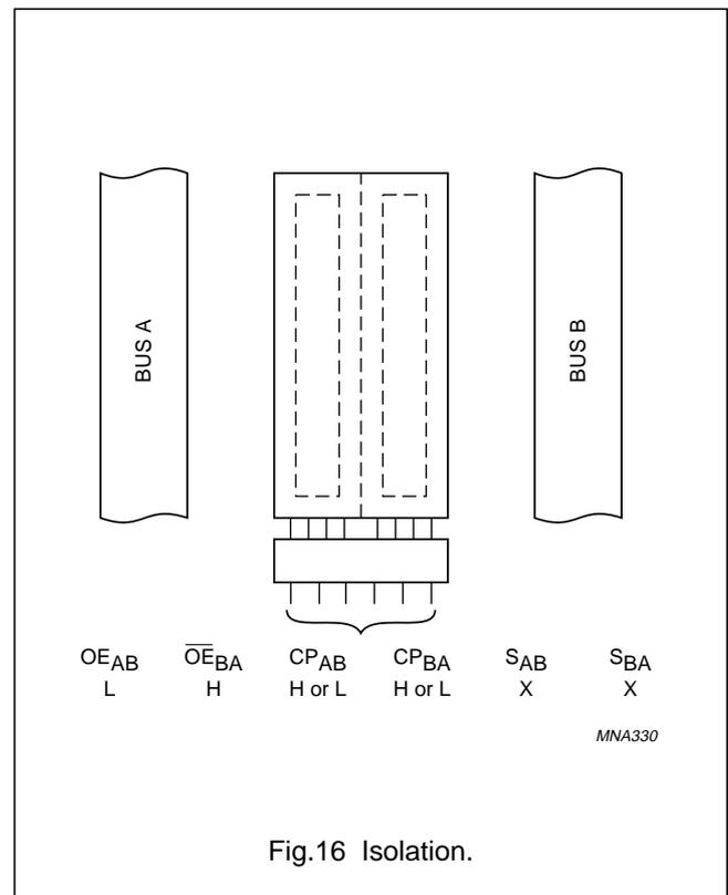
16-bit transceiver/register with dual enable; 3-state
