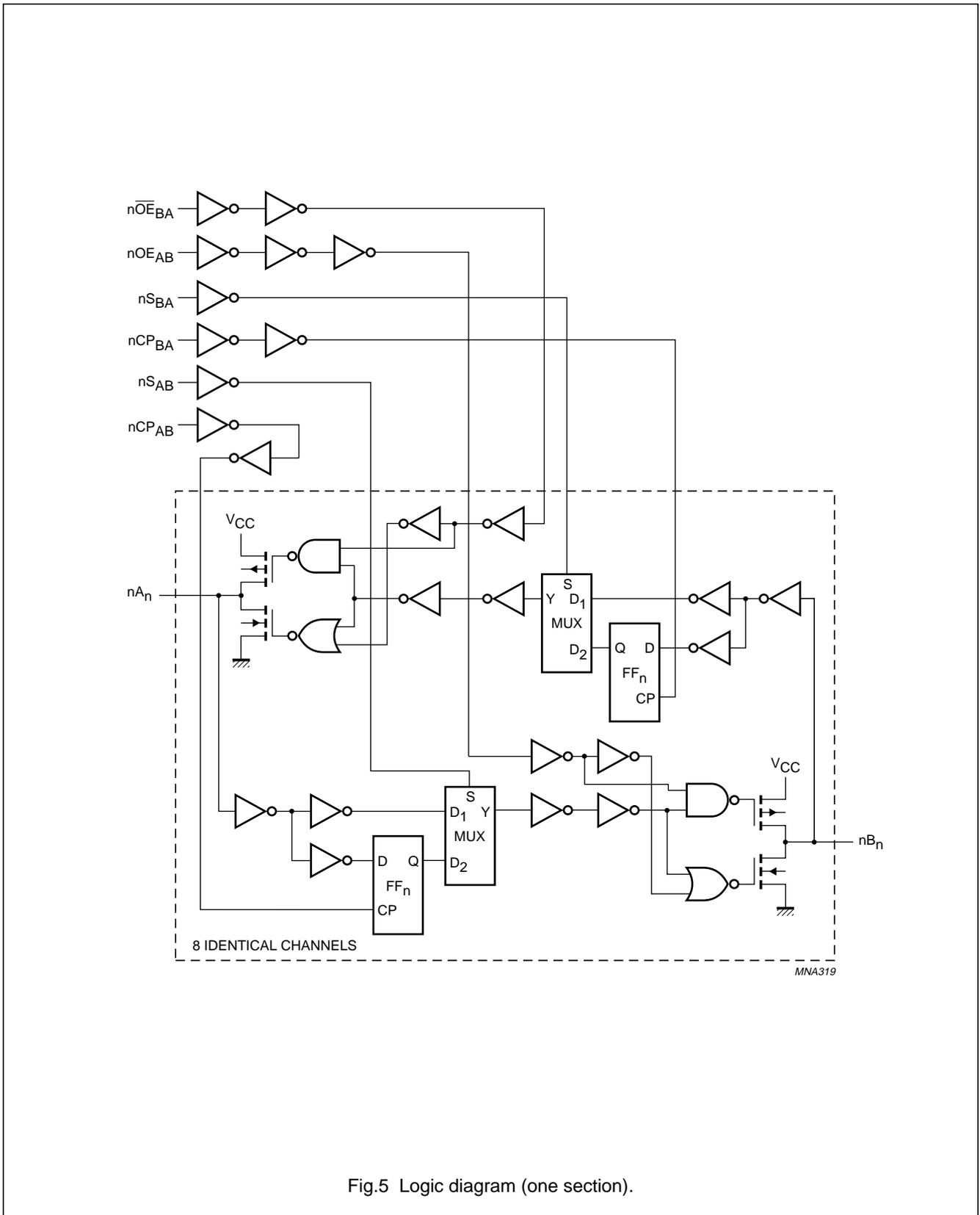
Fig.5 Logic diagram (one section).
