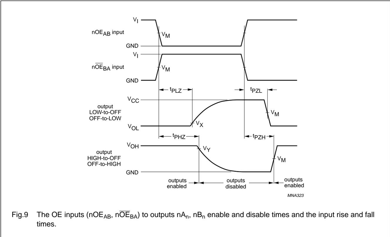
Fig.9 The OE inputs ( $nOE_{AB}$ ,  $nOE_{BA}$ ) to outputs  $nA_n$ ,  $nB_n$  enable and disable times and the input rise and fall times.
