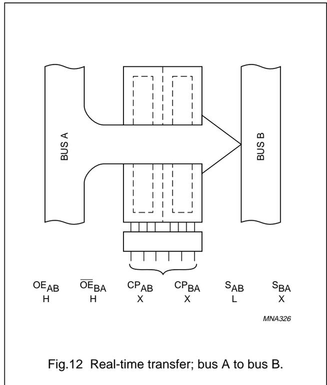
16-bit transceiver/register with dual enable; 3-state
