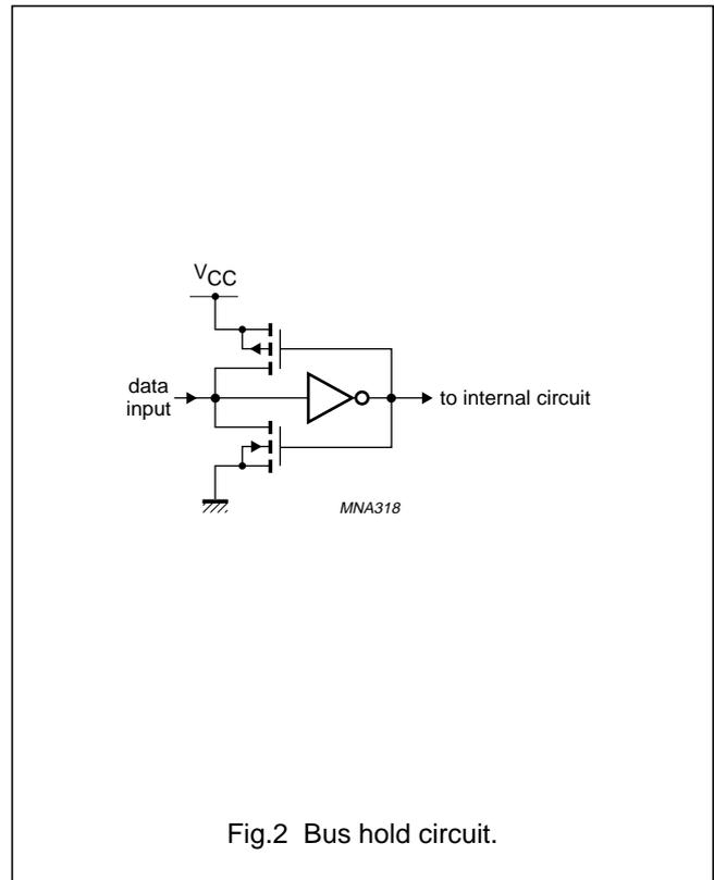
Fig.2 Bus hold circuit.
