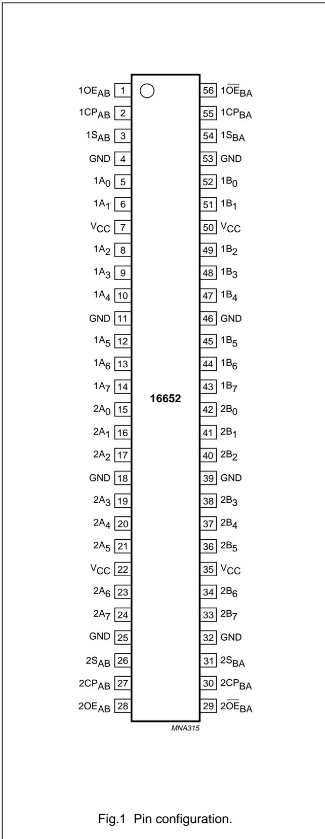
Fig.1 Pin configuration.
