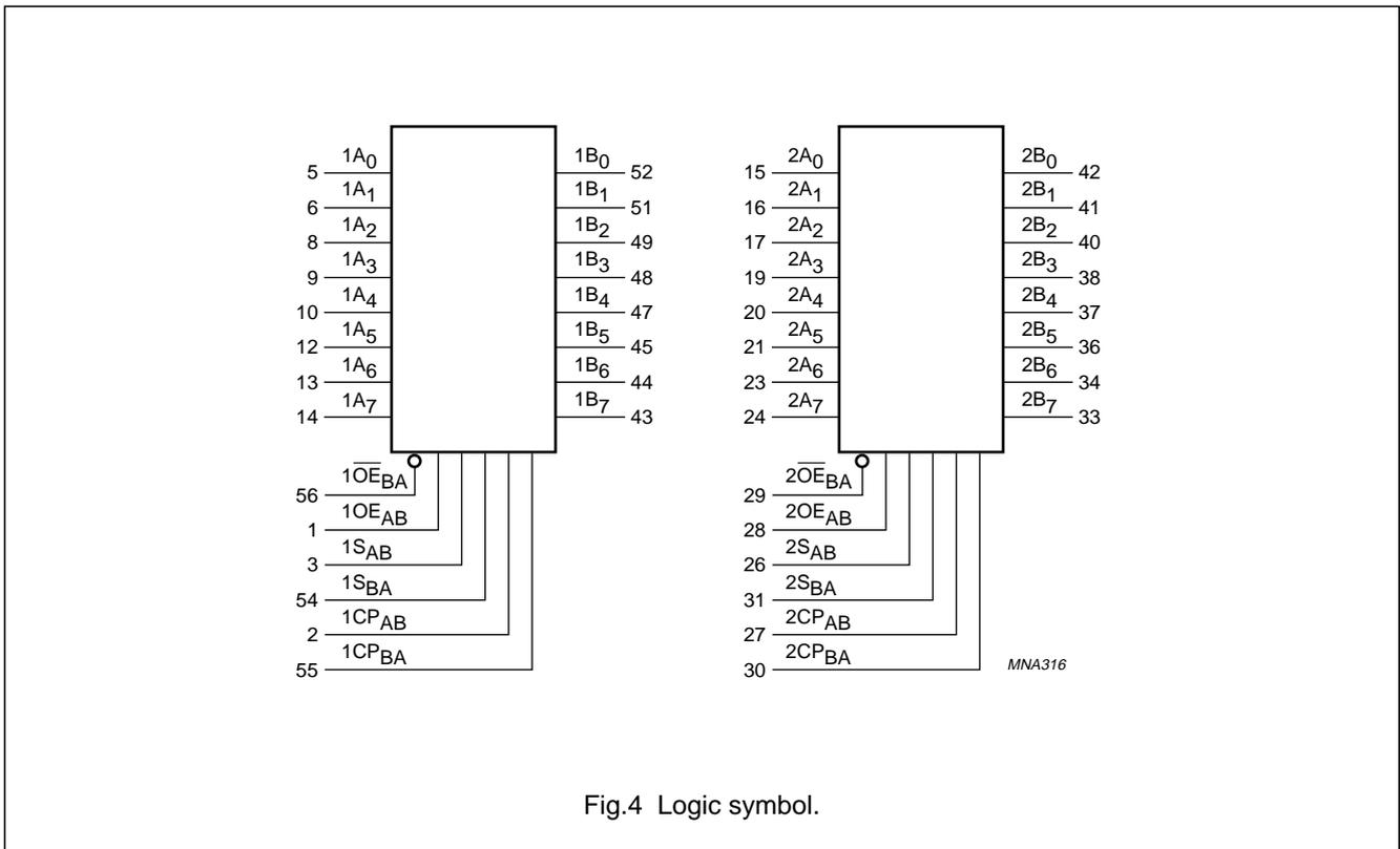
16-bit transceiver/register with dual enable; 3-state
