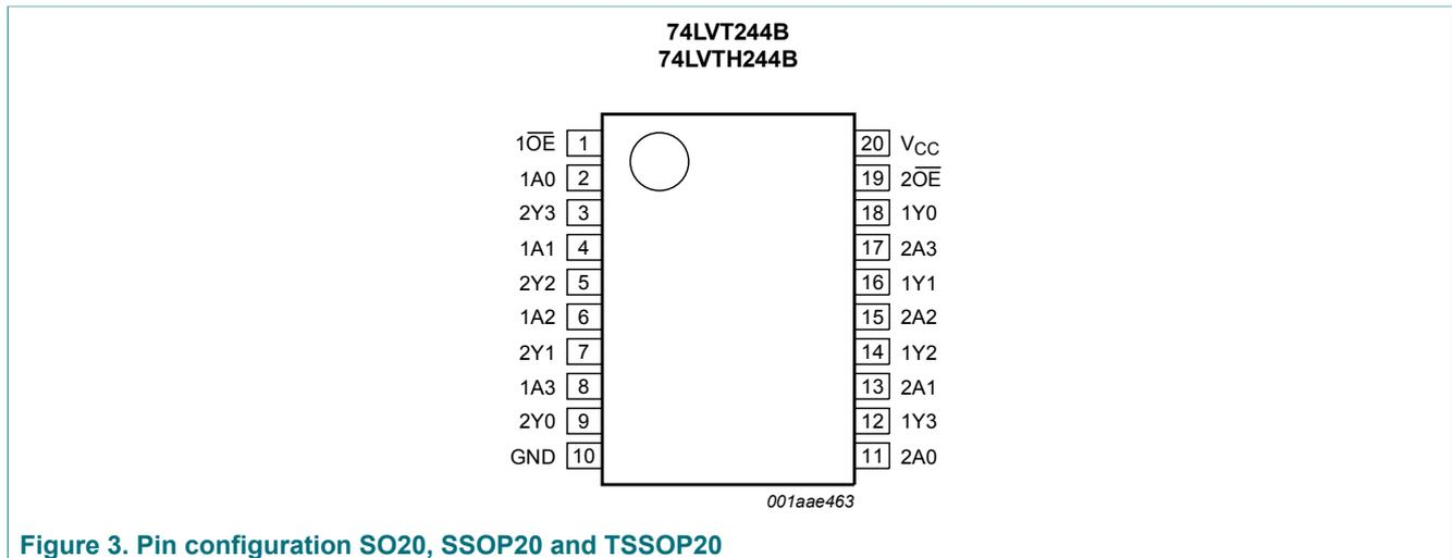
Figure 3. Pin configuration SO20, SSOP20 and TSSOP20
