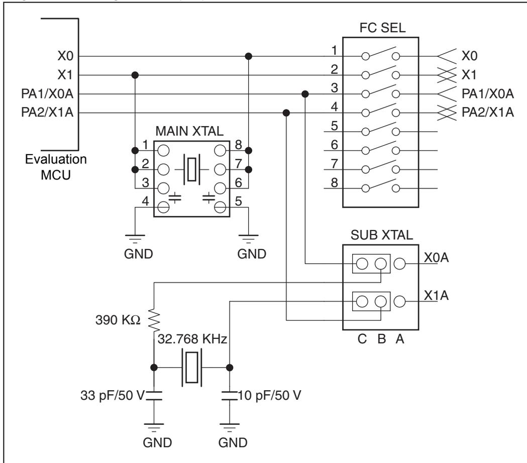
Figure 3-4. Examples of jumper settings for subclock selection
