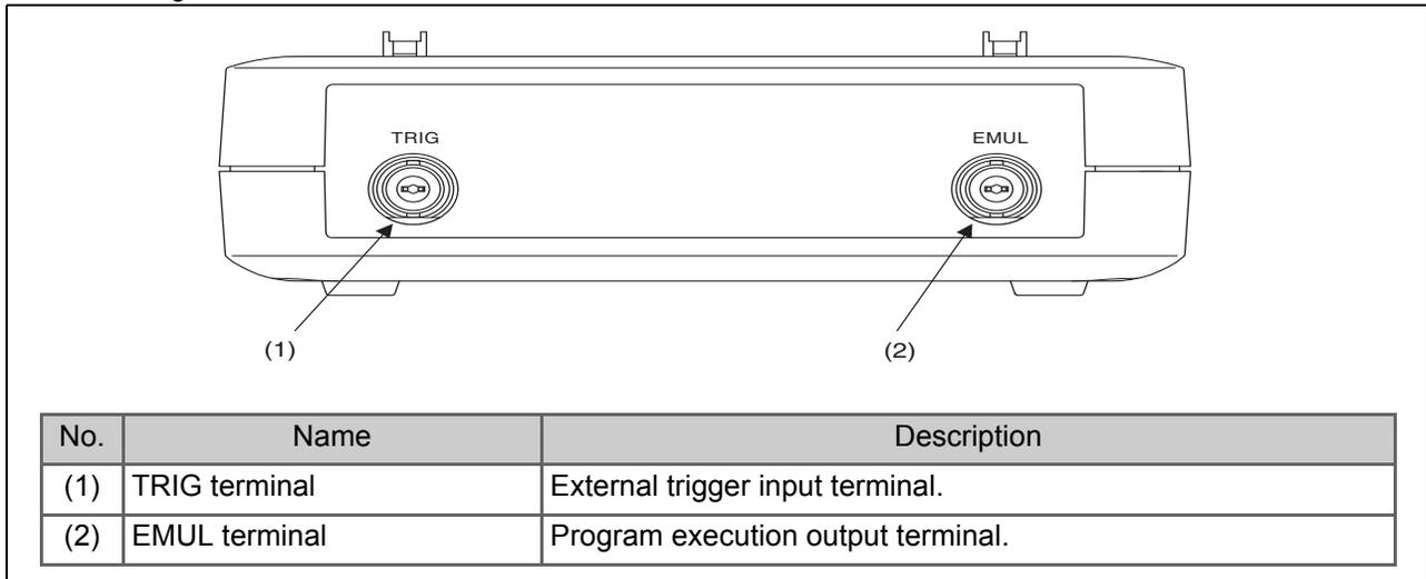
Figure 1-3. Rear view of the emulator unit
