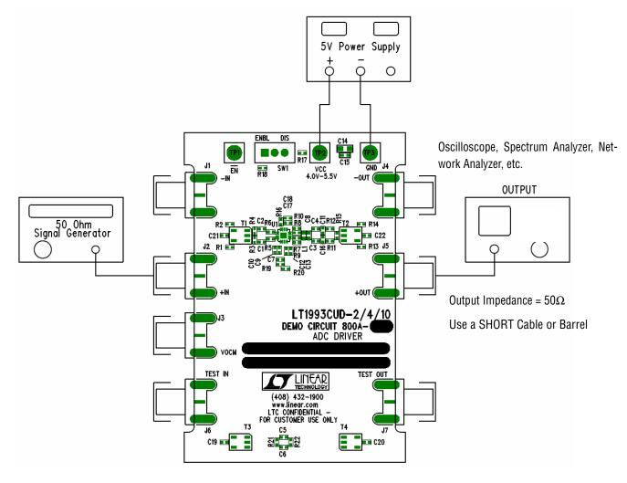
Figure 1. Proper Measurement Equipment Setup
