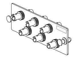
6 POSITION ST FIBER ADAPTER PANEL customer drawing
