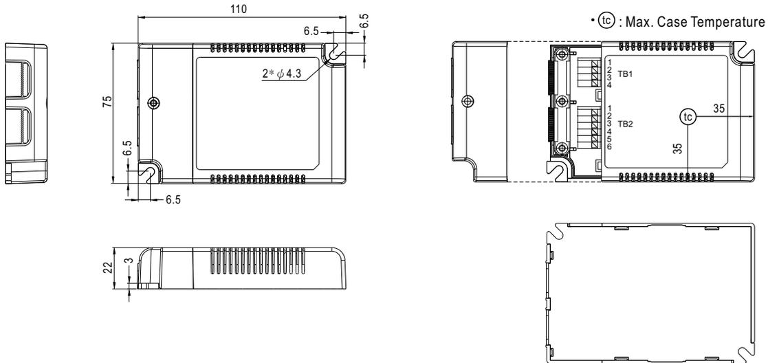
NOTE: Please use wires with a cross section of 0.75~1.5mm<sup>2</sup> for TB1 and wires with a cross section of 0.5~1.5mm<sup>2</sup> for TB2.
