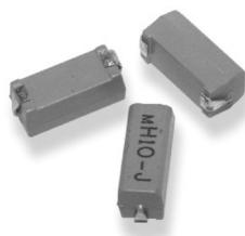
This is a high current, wound inductor, based on phenolic, iron or ferrite cores (depending on the value required). The terminations are of solder coated copper. Values from 0.1 $\mu$ H to 2.7 $\mu$ H have a phenolic core, 3.3 $\mu$ H to 100 $\mu$ H an iron core and 120  $\mu$ H to 1000  $\mu$ H a ferrite core.
