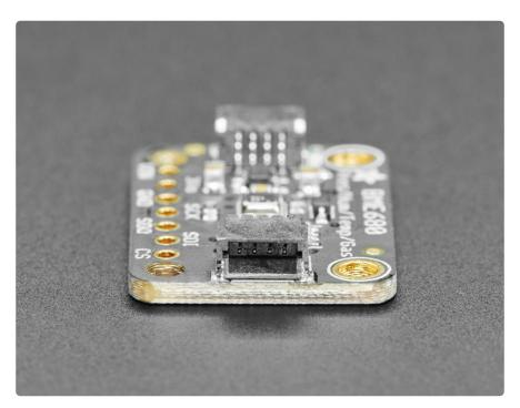
To make things easier and a bit more flexible, we've also included  $\underline{\text{SparkFun Qwiic}}$  () compatible STEMMA QT () connectors for the I2C bus so you don't even need to
