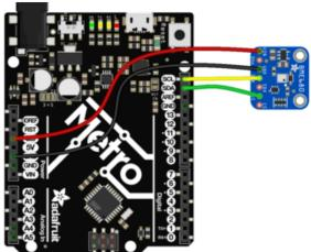
Connect Vin (red wire on STEMMA QT version) to the power supply, 3-5V is fine. Use the same voltage that the microcontroller logic is based off of. For most Arduinos, that is 5V. For 3.3V logic devices, use 3.3V
