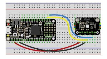
Board 3V to sensor VIN (red wire on STEMMA QT version) Board GND to sensor GND (black wire on STEMMA QT version) Board SCL to sensor SCK (yellow wire on STEMMA QT version) Board SDA to sensor SDI (blue wire on STEMMA QT version)
