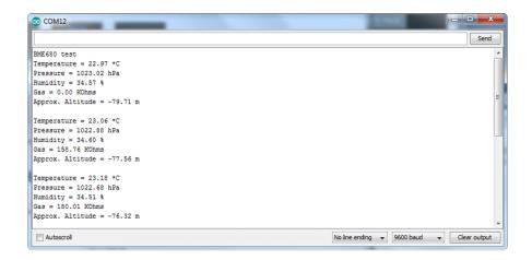
Temperature is calculated in degrees C, you can convert this to F by using the classic F = C \* 9/5 + 32 equation.
