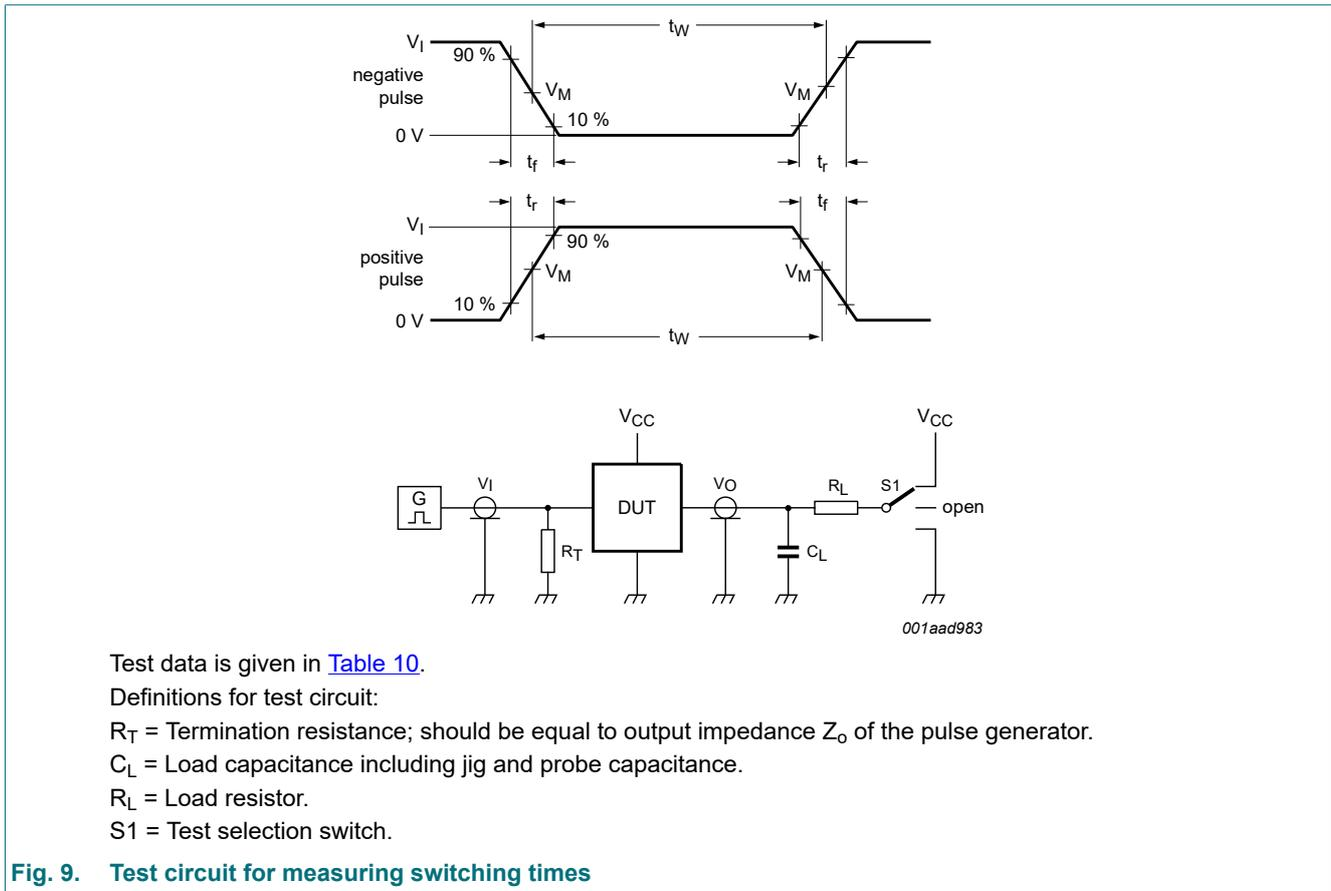
Fig. 9. Test circuit for measuring switching times
