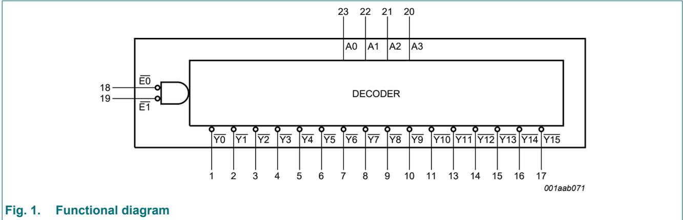
Fig. 1. Functional diagram
